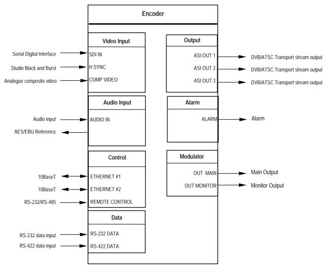
*Figure 2.8: Equipment Connections for the Basic Unit*
